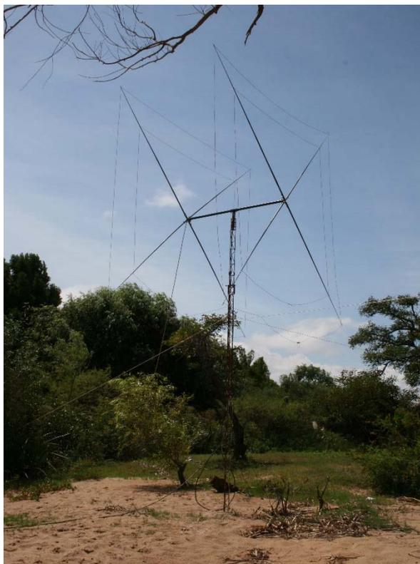
A 14AVQ vertical mostly to be used on 20m, was put on the small beach where we had landed. For 17m, a delta loop was hang up in a tree and a inverted V dipole for 12m (CX3AN made) with the apex at only 4m above ground was hang up from another tree. Gustavo-CX2AM had made a shack (height 2m, wide 2m, length 3m) entirely made of mosquito nets. The shack had a cover against the rain fixed at four points to trees.
