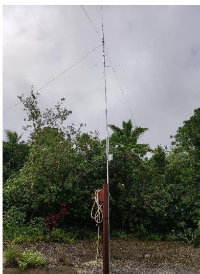
GP7 multiband vertical designed and manufactured by SP7GXP
