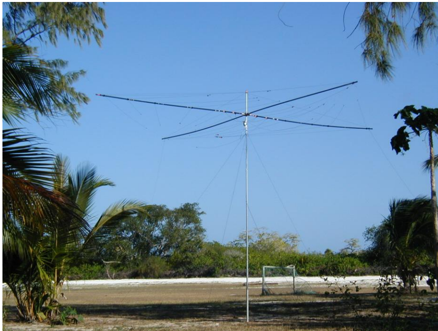
The Five bands Spiderbeam, heading Asia
