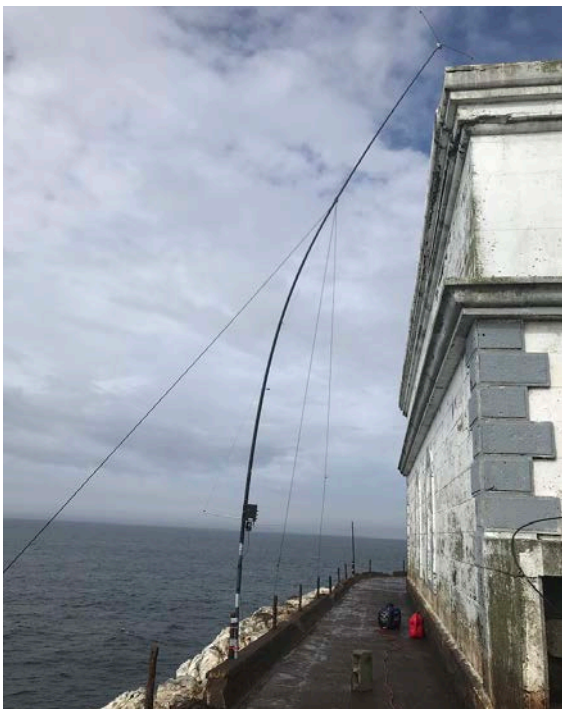
Crank IR vertical was used on 17 and 40 m
